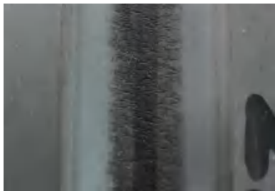
The surface quality of regular grades after one shift of rolling
